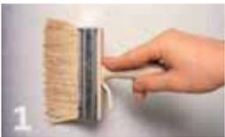
The surface must be consistent, flat and clean. It must be dry and free of grease. If the surface is porous then apply first a layer of Cemix Primer. Allow to dry for 2 hours and then you can begin.
